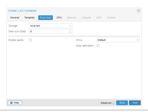
The root mount point is configured with the rootfs property, and you can configure up to 10 additional mount points. The corresponding options are called mp0 to mp9, and they can contain the following setting:
