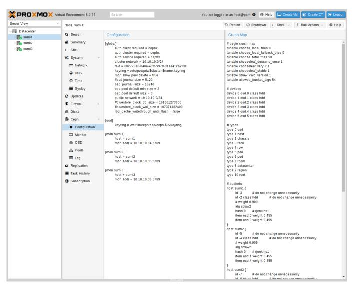
After installation of packages, you need to create an initial Ceph configuration on just one node, based on your network (10.10.10.0/24 in the following example) dedicated for Ceph:
