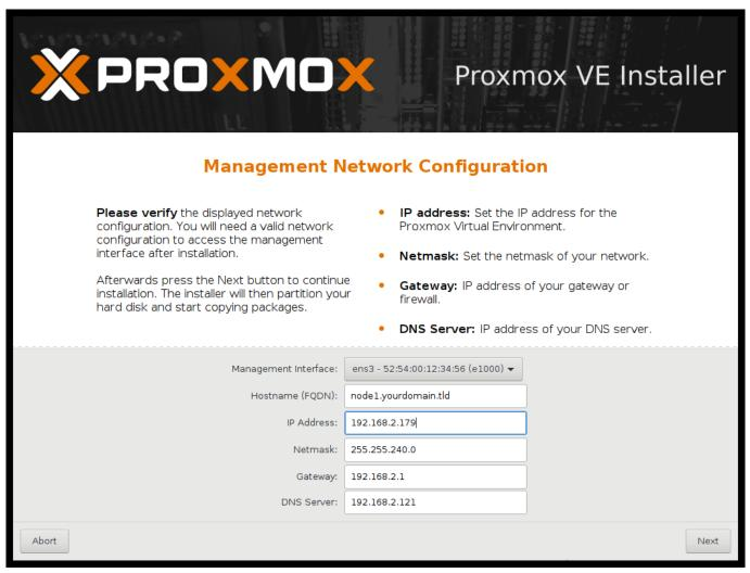
The last step is the network configuration. Please note that you can use either IPv4 or IPv6 here, but not both. If you want to configure a dual stack node, you can easily do that after installation.
