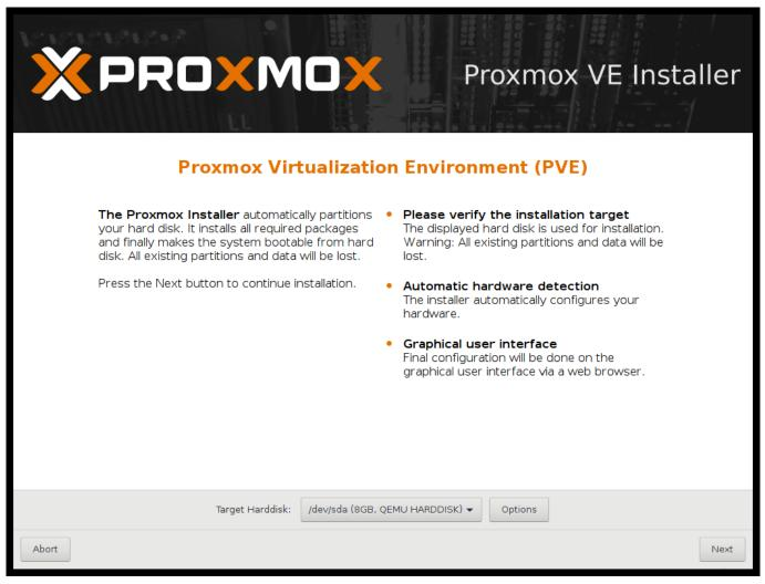
You normally select **Install Proxmox VE** to start the installation. After that you get prompted to select the target hard disk(s). The Options button lets you select the target file system, which defaults to ext4. The installer uses LVM if you select ext3, ext4 or xfs as file system, and offers additional option to restrict LVM space (see below)
