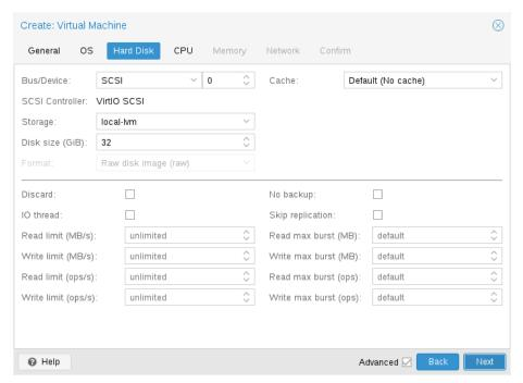
On each controller you attach a number of emulated hard disks, which are backed by a file or a block device residing in the configured storage. The choice of a storage type will determine the format of the hard disk image. Storages which present block devices (LVM, ZFS, Ceph) will require the **raw disk image format**, whereas files based storages (Ext4, NFS, CIFS, GlusterFS) will let you to choose either the **raw disk image format** or the **QEMU image format**.
