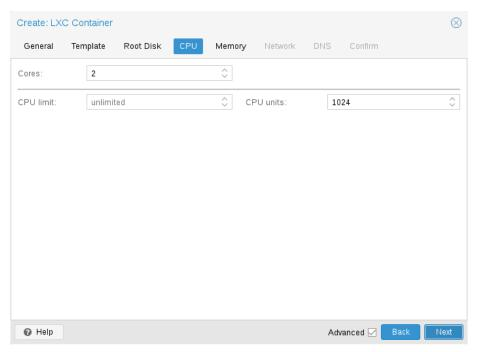
You can restrict the number of visible CPUs inside the container using the cores option. This is implemented using the Linux *cpuset* cgroup (**c**ontrol **group**). A special task inside pvestatd tries to distribute running containers among available CPUs. You can view the assigned CPUs using the following command:
